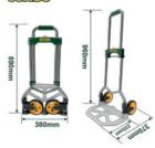
Load capacity: 60kg Material: steel pipe and steel foot plate Extended size: 370x380x960mm Folded size: 380x55x690mm Foot plate size: 235x380mm Wheel diameter: 130mm (PP+silent TPR plastic) Including elastic bungee cord Compact design - easy to store almo
