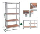
5-Tier adjustable storage shelves Product size: W700mm x D300mm x H1500mm Each shelf load capacity: 175kgs (place goods must be evenly) Material: MDF board & galvanized steel frame
