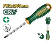
Tip type: Phillips Tip size: PH3 Round shank Diameter: 8.0mm Length: 200mm Material: Cr-V steel Blade finish: black tip Magnetised tip Comfortable soft grip handle Packed by plastic hanger
